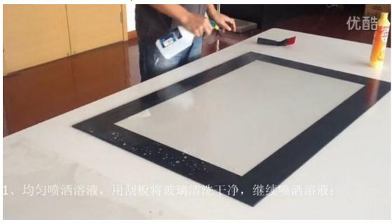
3) Tear off the protective film from permanent type touch film. When you are tearing off,please spreading the soap water to the touch film(把背胶版触摸膜保护膜撕开,边撕边喷洗洁精水到触摸膜上)
