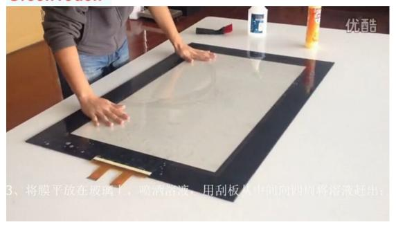
5) After Position the touch film perfectly, Spread the soap water to the glass(触摸膜位置选好后,往触摸膜上喷洗洁精水)
