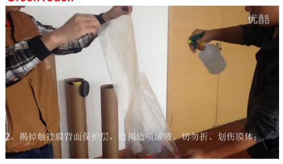
4) After the protective film is teared off,place touch film on the glass.(保护膜撕去后,将触摸膜放置在清洗后的玻璃上)
